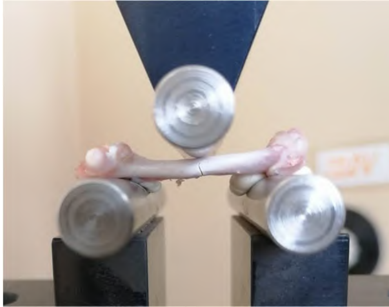
Figure 4. The process of preparing bone tissue for biomechanical strength testing.
